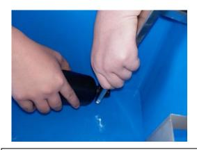
Step 5: Remove the secondary filter as shown in the following two figures.
