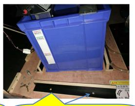
Step 3: Remove this wood block and pull out the Water Tank a little bit.
