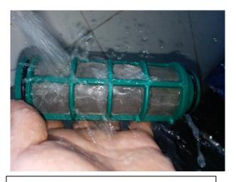
Step 7: Remove the filter element and rinse with tap water until the dirt is flushed.
